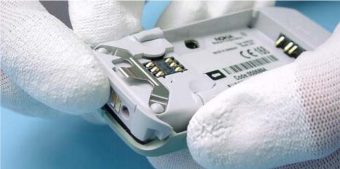
Take care that your workbench is always clean and protect the Window with a foil against dust and scratches. Release the A-Cover from the bottom side of the unit.
