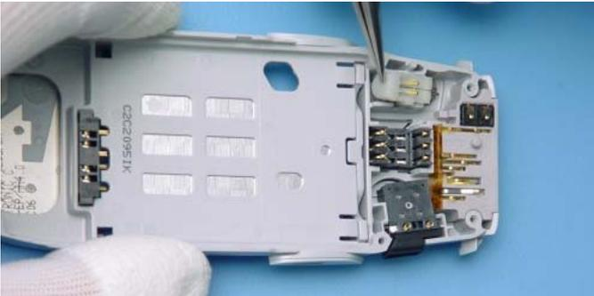
The Vibra Motor with its rubber housing is pressed into the D-Cover.
