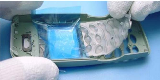
Also, protect the inner part of the window with a foil. The Keymat is loose inside the cover.
