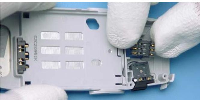
Remove the SIM Connector by hand. Note the right direction, when replacing the SIM connector. It only fits in one direction.
