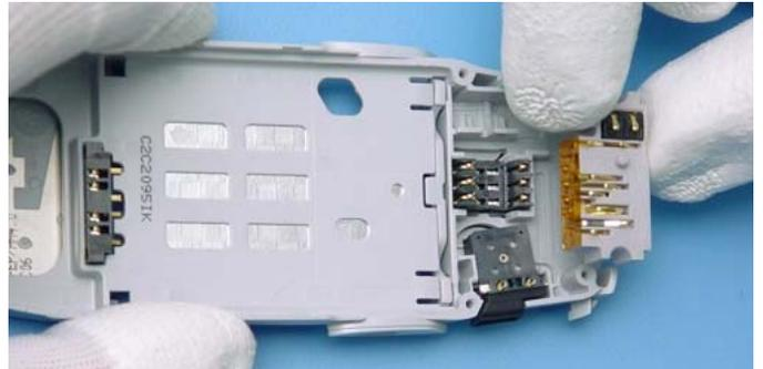
No special tools are needed to remove the System Connector. Note that the Microphone cannot be changed separately (like in other products), because it is one unit with the System Connector.
