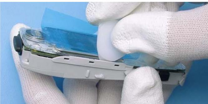
When releasing the side clips of the D-Cover you can use plastic tweezers or the opening tool from 5510 (SRT-6, 0770431), as shown in the picture.
